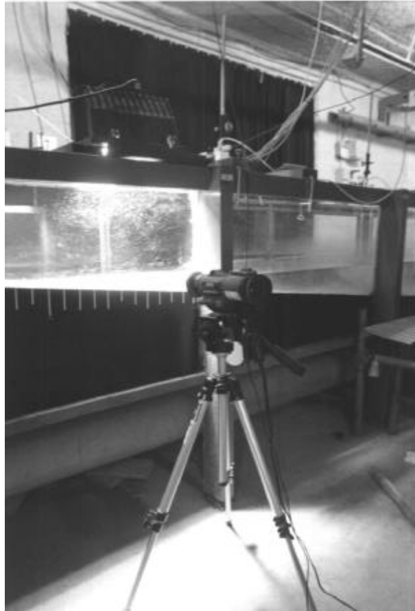
Fig. 2.11 - Videocamera of the Image analysis system.
