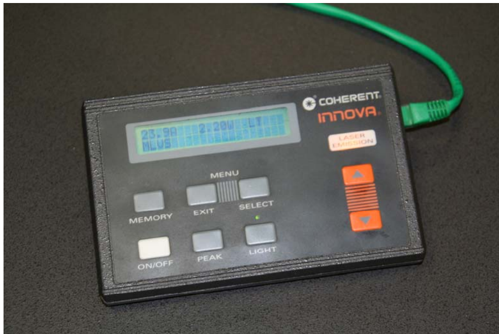
Figure 6. Current flowing and overall power of the laser during running tests. LT means that a light intensity feedback control has been selected
