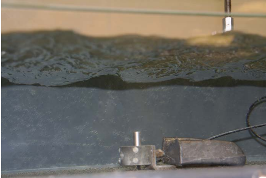
Figure 28. Ultrasound Doppler Velocimeter probe set-up
