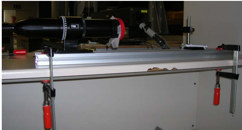
Layout of the probe and microscope on a board clamped to the table
