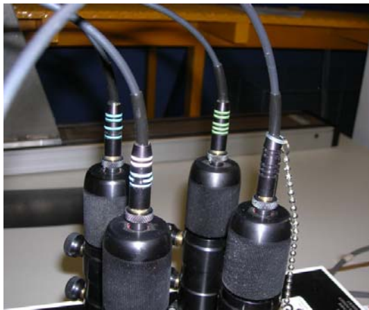
(a) Alignment check cable and (b) TSI connector of the check alignment cable inside the green shifted shutter.
