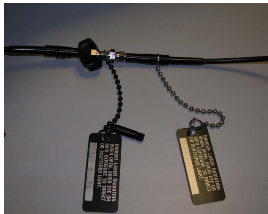
Connection of the receiving fibre to the check alignment cable.
