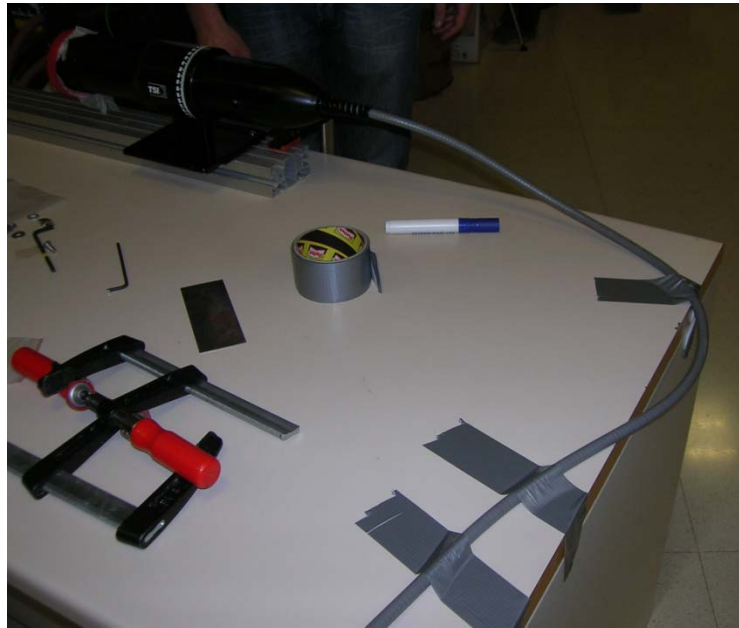
Fastening of the cable to the table.
