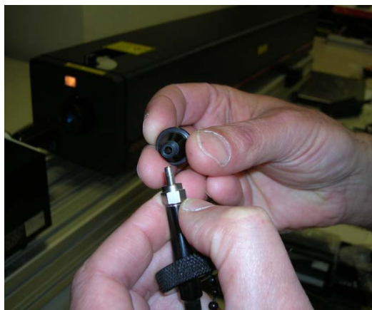
Removal of the connector at the end of the receiving fibre.
