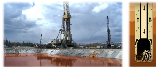
Drilling fluid (mud): in mining engineering, it is used to aid the drilling of boreholes into the earth.
