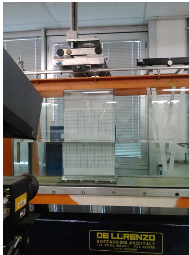
Figure 29. Calibration mesh suspended in the flume in the sheet light of the laser
