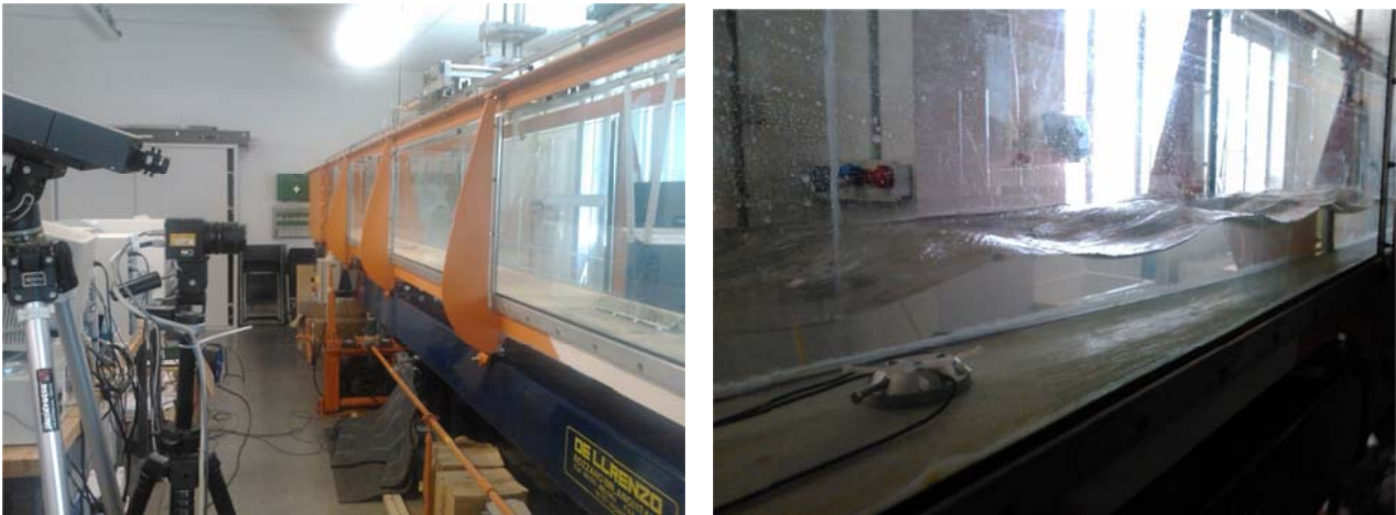
Figure 4. Laser and camera for the PIV (left), and UDVP placed on the bottom (right)
