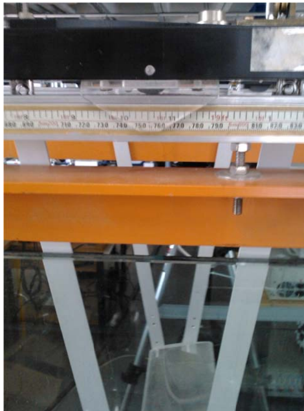
Figure A1. Rule in the upper part of the flume
