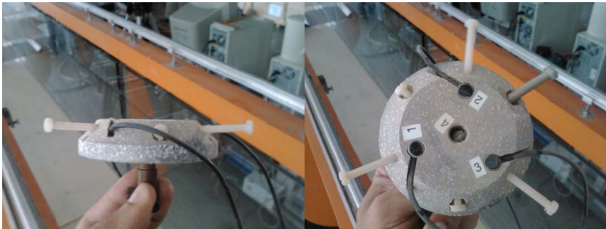
Figure 7. Disposition of the transducers. View from side and above.
