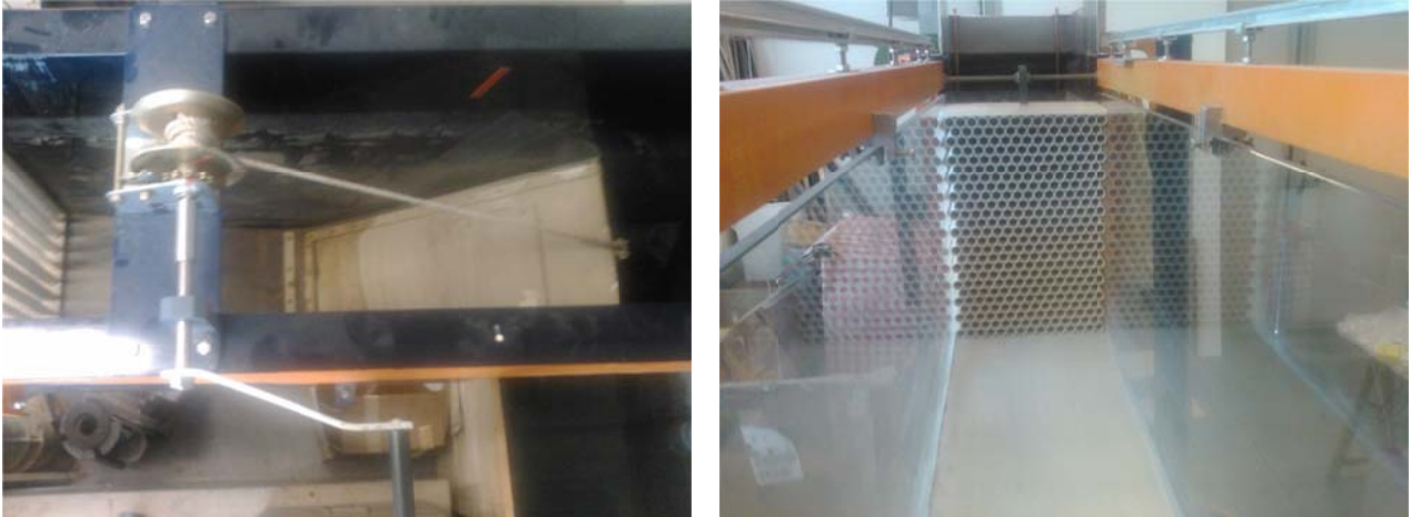
Figure 1. Bottom hinged flap gate (left) and the flow straightener in the flume (right)
