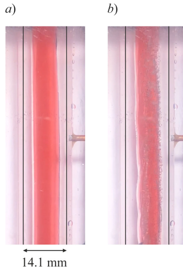
Figure 3. Evolution of the radius of the internal fluid due to a sudden reduction of density. Vertical pipe with internal radius R = 7.05 mm. a) Initial configuration, with \rho_a = 1225.3 \text{ kg/m}^3 , \rho_d = 1257.7 \text{ kg/m}^3 , \mu_a = 10^{-3} \text{ Pa s} , \mu_d = 0.329 \text{ Pa} , Bm_a = 0 , Bm_d = 0 and \delta_0 = 0.65 . b) Configuration after reducing the ascending fluid density, with \delta_1 = 0.56 . The ascending fluid is glycerol plus water, the internal fluid is water added with phosphates, sodium chloride and citric acid. The injected fluid is water added with phosphates, sodium chloride and sodium bicarbonate having the same density of the internal fluid.
